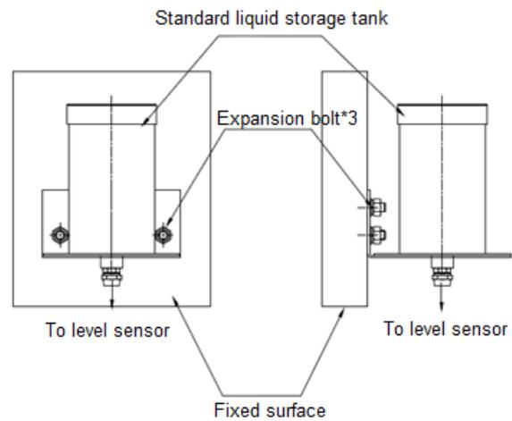
**Standard liquid storage tank installation diagram**
