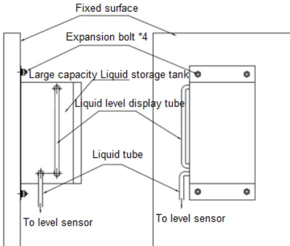
**Large capacity liquid storage tank installation diagram**
