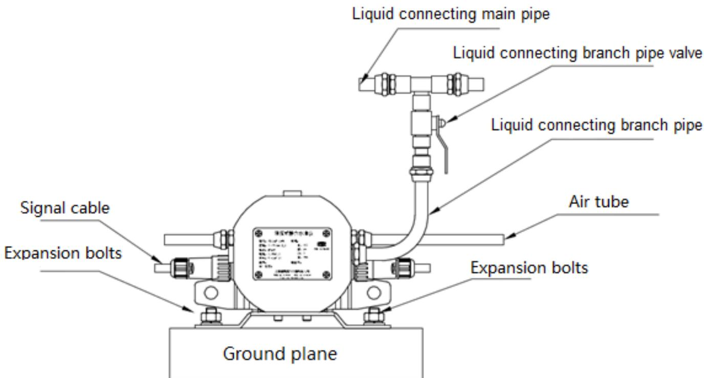
**Flat mounted : Screw-fixed type diagram**
