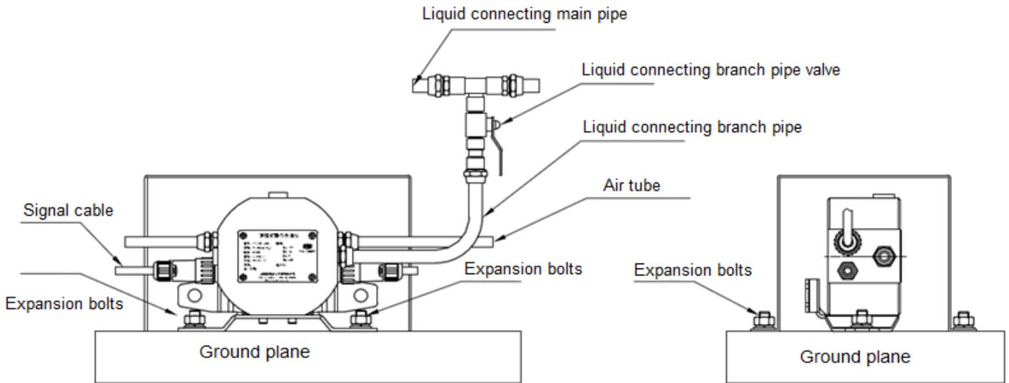
**Flat mounted : Protective box integrally bonded type diagram**
