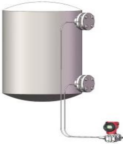
Tank Liquid Level Measurement
